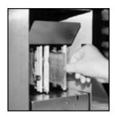
Rear lint screen cleaning. When visibly dirty, remove the lint screen from the back of the unit and flush it with hot water. Remove the glass ozone plate(s) by grasping the plate's center edge nearest you and pulling straight out.
