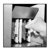
Dry completely, using a hair dryer if necessary. Reinstall ozone plate. Be sure to check that the electrical tabs are in contact with the plate.
