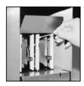
Also be sure to clean the white standoffs which make up the legs of the ozone plate card cage (a cotton swab with alcohol works well).
